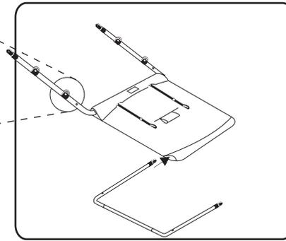
**6** Position Bow 2 as shown with holes facing up. Thread Bow 2 through front sleeve of fabric.
