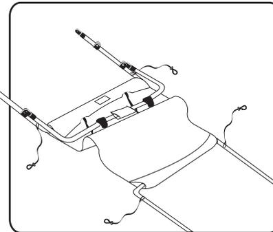
**10** From the Bow 1 jawslide nearest to Bow 3, remove screws to attach eye end of Bow 3. Eye ends will rotate to line up. Resecure with screws as shown.
