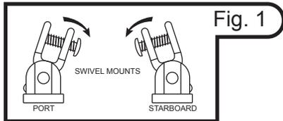
**12** Determine what area of the boat you want to cover with the bimini. Bimini swivel mount locations are approximately half the distance of the total length of the bimini. Measure for mount placement and mark. Make sure the swivel mounts are parallel to each other and facing with the swivel movement going toward inside of boat (See Fig.1).
