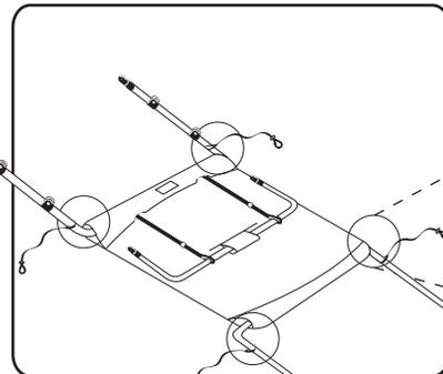
**8** Pass looped end of each hold down strap over end of bow.
