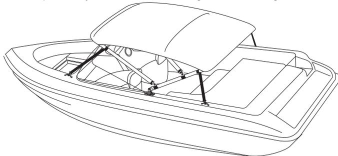
**13** With bimini secure in the mounts, open the bimini and determine the best position for the hold down strap eyes. Strap eyes should be mounted to a flat surface whenever possible and straps should maintain an angle between 30 and 60 degrees from front to rear. To minimize side to side movement, it is suggested to mount front strap eyes as far inboard as allowable. Line up strap eyes across the boat.
