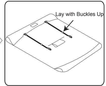
**4** Insert bow straps into cutout of rear sleeve as shown. Leave straps fully extended.
