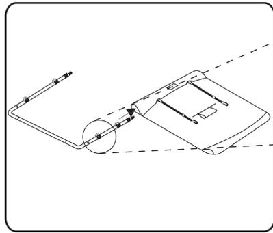
**5** Position Bow 1 as shown with jaw slides facing up. Thread Bow 1 through rear sleeve and bow strap loops.
