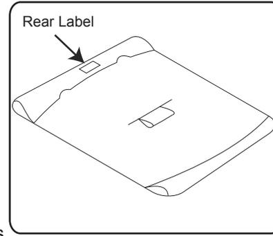
**3** Lay bimini fabric face down on a flat clean surface (label on rear sleeve will be facing up)
