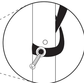
**9** Line up hole in each strap with the hole in the bow. Insert #8x1/2" screw through washer and strap, and secure into bow. Strap should extend away from the top. Repeat for remaining bow straps.
